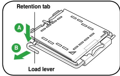
3. Lift the load lever in the direction of the arrow to a 135° angle.
