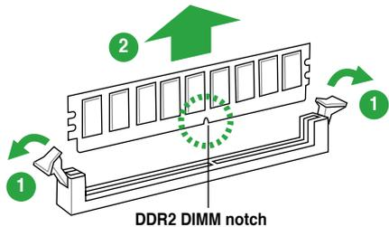
2. Remove the DIMM from the socket.
